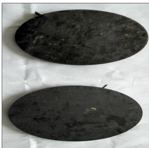
Figure 9. Testing specimen for thermal conductivity
